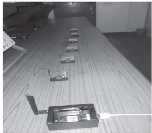
Figure 3. WSN nodes deployed inside the building.
