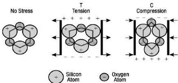
Figure 2. Mechanism of piezoelectric effect in quartz crystal.
