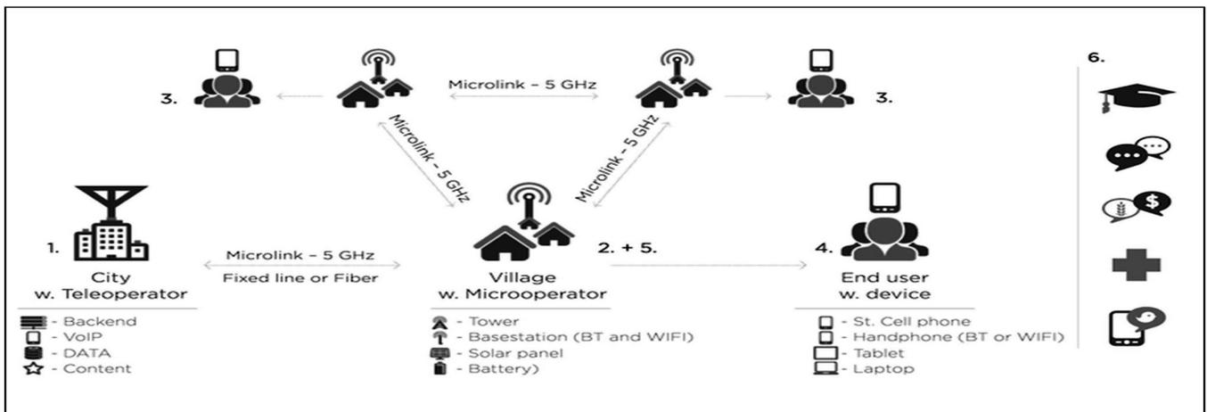
Figure 2. Communication-solution deployed in rural areas of Africa.
