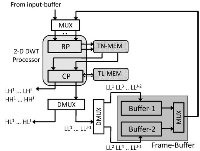
Figure 1. General structure for line based 2-D DWT.
