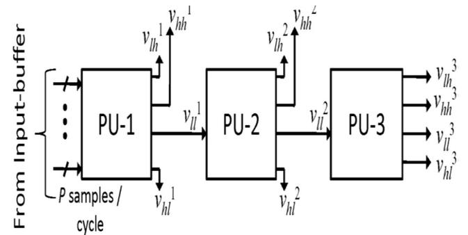
Figure 4. Computation structure for three level 2-D DWT.
