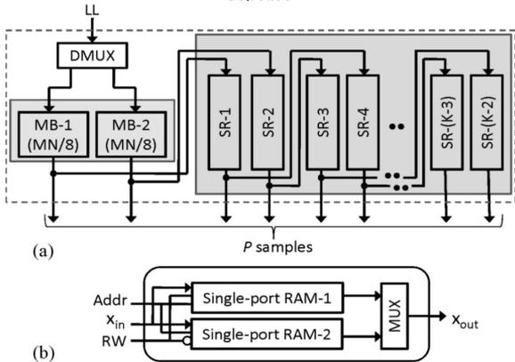
Figure 3. Structure of Buffer-1 and SR using single-port RAM. The size of upper high and upper low (UL, UH) intermediate matrix forms a pair. In the processing from transposition memory first, column processor receives the (UH and UL) components in the counter clock wise direction and then it generates the four sub-band matrix of signal after decomposition  $[LL^1, LH^1, HL^1 \& HH^1]$  of size of  $(M/2 \times N/2)$  Matrix at each cycle.
